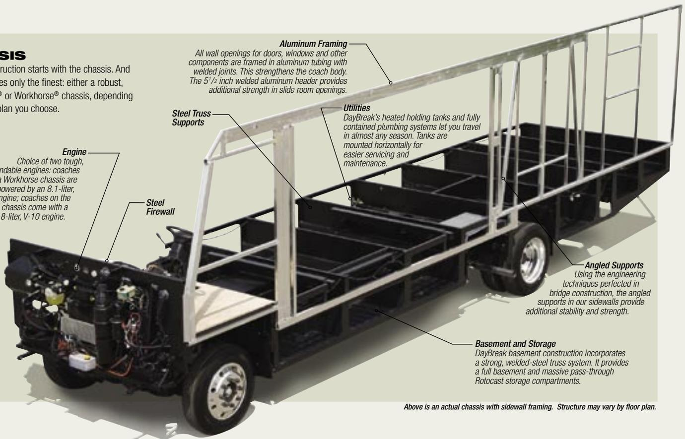
Above is an actual chassis with sidewall framing. Structure may vary by floor plan.
